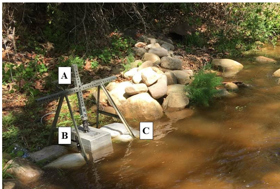
FIGURE 3. Carpinteria Creek DIDSON deployment infrastructure with key features labeled. (A) A-frame; B) DIDSON housed in a debris box and silt box; (C) gravel bags anchoring sled feet.
