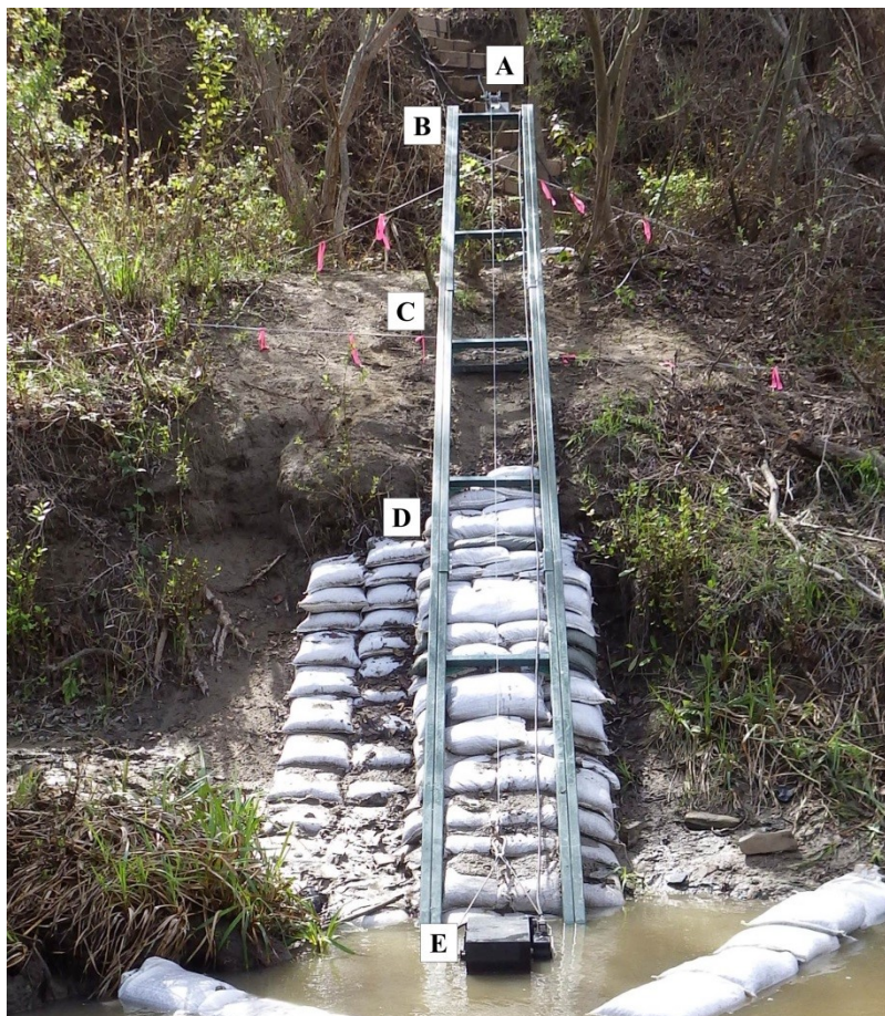
FIGURE 2. Salsipuedes Creek DIDSON deployment track system as seen during its last deployment in 2014 with key features labeled. (A) winch; (B) track; (C) cross-bracing cables; (D) gravel bag berm; (E) DIDSON/X 2 /sled assembly.
